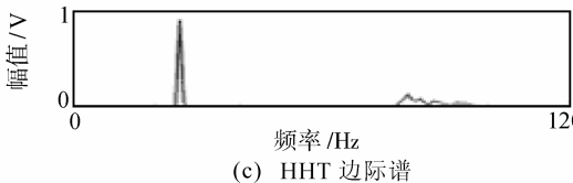
图4 仿真信号HHT变换 Fig. 4 HHT of simulation signal
