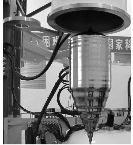
图7 cusp磁场环境下生长的单晶 Fig. 7 The growing single crystal under cusp magnetic field condition
