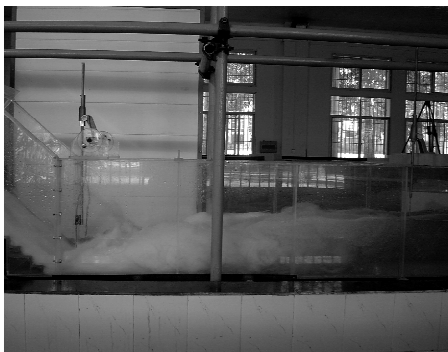
图 3 临界水跃时消力池内水流掺气现象 Fig. 3 The air entrainment of the stilling basin when critical hydraulic jump
