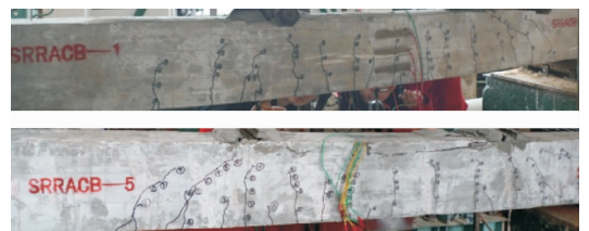
图1 型钢再生混凝土梁受弯典型破坏特征 Fig. 1 Typical flexural failure characteristics of SRRACB concrete beams
