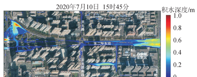
图 5 西安市二环北路明珠家居至未央立交段模拟内涝积水 Fig. 5 Simulated inundation of the region between Mingzhu furniture store and Weiyang overpass, Xi'an Erhuan North Road
